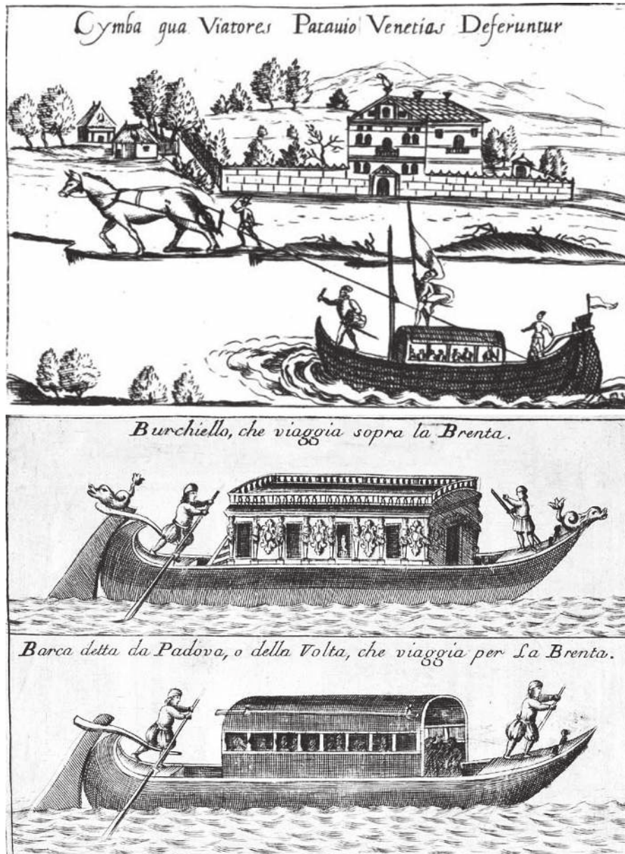
Figure 10: Top: The Barca da Padova in 1591, towed by a horse along the Brenta. Passengers can be seen seated on two benches, facing each other. Bottom: 18th Century engraving depicting (top): The Burchiello, with its wooden cabin and balconies and (bottom): the Barca da Padova, the public ferry.
