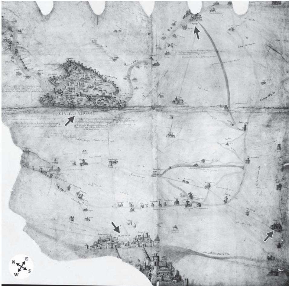
Map 4: from the late 1470s or early 1480s. Veronese territory. Verona is in the upper left quadrant, Legnago in the upper right, Mantua at the bottom, the Po along the right edge. Despite the distortions in scale and orientation, a canal is clearly shown connecting Legnago to the Tartaro at La Crocetta, labeled “fossa fexe far el ducha de milan,” thus dating it between 1387 and 1402. In 1482 this canal was filled in for military reasons. Upper right: the (much fainter) Castagnaro. Lower right: the Tartarello branching out from the Tartaro at Bastion San Michele; the Tartarello was used for navigation before the Fosssetta mantovana was dug (end of the fifteenth century). At Tor de mezo, the Tartarello meets the straight line running from Ostiglia (extreme right) to Ponte Molino (on the Tartaro branch); this line likely represents the Via Claudia Augusta to Verona and/or the parallel Fossa d’Ostiglia. (ASVe, Scuola di S. Maria della Carità, b. 36, n. 2530)
