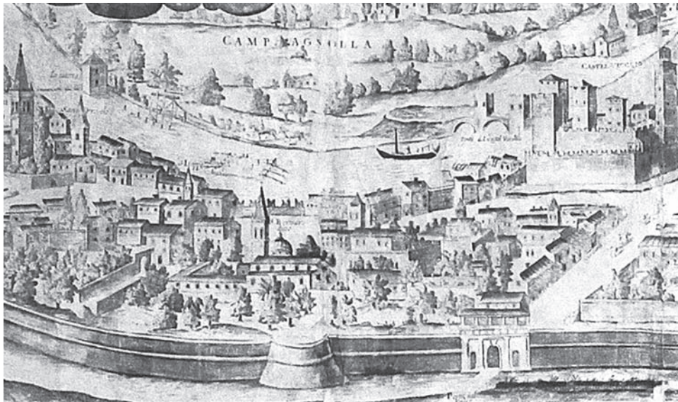
Figure 2: The Adige enters Verona. Upper left: the chain and tower La Catena; an irrigation waterwheel; horses towing a burchio upstream, just past the Ponte Castelvevchio; and a descending timber raft. Bottom: the western fortifications with the Porta Palio. (Detail from Verona città celebrima of Paolo Ligozzini (1620), BCVr, Stampe 1.b.18)
