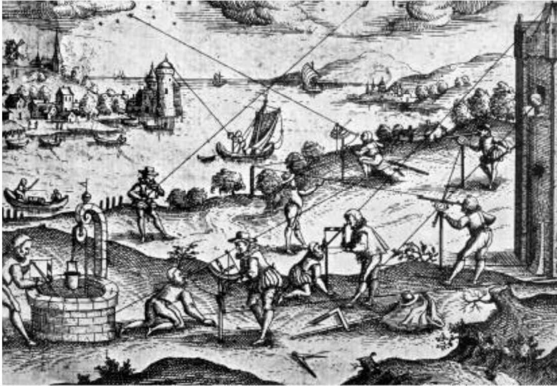
Amateur astronomers of the late sixteenth century at some unknown location, probably in Germany or the low countries (the engraving is from the Deutches Museum in Munich). Although no details of time and place accompany this engraving, art historians can infer the date—"late sixteenth century"—from the costumes. The instruments depicted are obviously a variety of tools for measuring distance and examining objects at a distance, while several appear to be telescopes. The numerous figures attest to the excitement and popularity surrounding the new vistas that such instruments were opening at this time.
